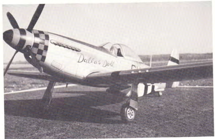
PS/D Mustang. Built from scratch. Hand made fiberglass spinner and cowl. Hand made retractable landing gear.
