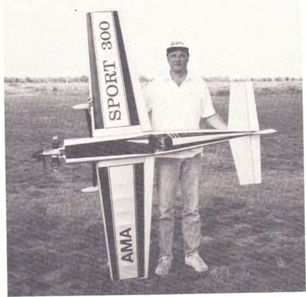
Sport 300, 7 feet by 6 feet, 60 mph maximum speed. Cost $1800 and took 2 weeks of spare time to build.
